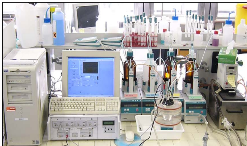
High precision potentiometric titrator with ionic strength control
