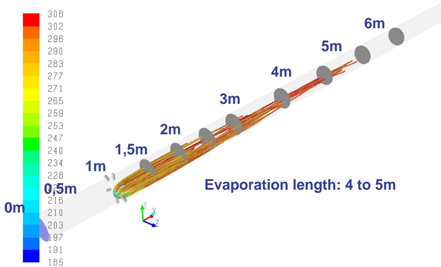
Discrete Particle Model without coalescence or break-up.
